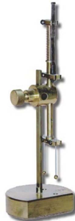
FIGURE 24: THE TECHNIQUE FOR THE LOCALISATION OF PROJECTILES IN THE EYE. A TUBE SHIFT METHOD IS USED WITH TWO RADIOGRAPHS AND THE W. SWEET DEVICE (SEE DETAIL VIEW).
