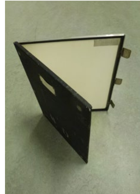
FIGURE 7: TRADITIONAL X-RAY FILM CASSETTE WITH INTENSIFYING SCREENS.
